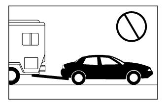
Notice: Towing your vehicle from the rear could damage it. Also, repairs would not be covered by the warranty. Never have your vehicle towed from the rear.
